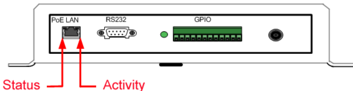
Figure 3: Network Status and Activity LEDs
